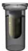
Stage 1 - Boiling Boiling solvent is covering the sample so that extractable material can be liberated.
