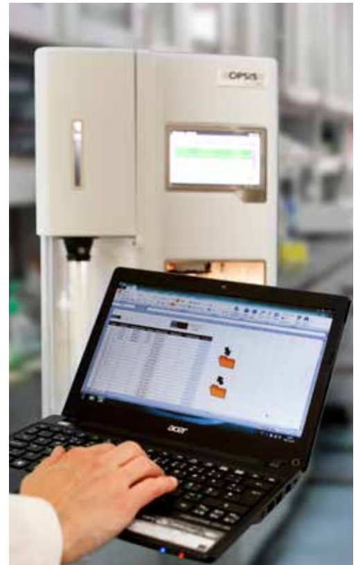
THE KJELROC OPEN FORMAT MAKES IT EASY TO USE A SPREADSHEET PC PROGRAM WITH AUTOMATIC TRANSFER OF WEIGHTS AND RESULTS TO/FROM THE INSTRUMENT.
