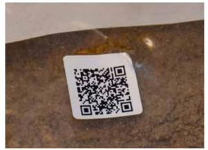
USE A LABEL PRINTER TO PRINT QR CODES FROM LABCONNECT. THIS WILL SIMPLIFY SAMPLE TRACEABILITY.
